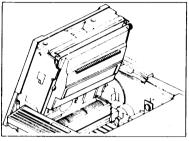
2. While holding down the green master unit release lever, slide out the master unit (lift the green ledge as shown in the diagram).
